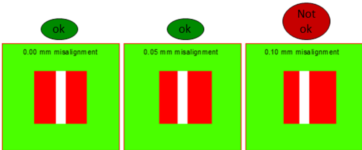
Figure 6. Diagram above shows the level of misalignment between the solder mask (green, for illustration only) and copper trace pattern (red). From left to right: no misalignment, 50 \mu m misalignment and 100 \mu m misalignment which will result in the left copper pad having 40% less exposed copper area than the right pad.
