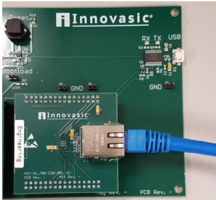
*Figure 6 – Ethernet Personality Module Connection*
