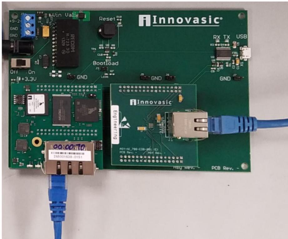
Figure 9 – Assembled TSN Gateway with Connections
