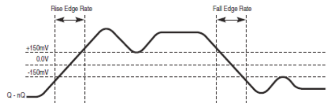
DIFFERENTIAL MEASUREMENT POINTS FOR RISE/FALL TIME
