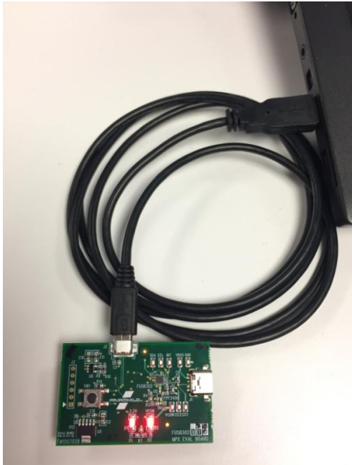
Figure 2 - EVB powered from PC
