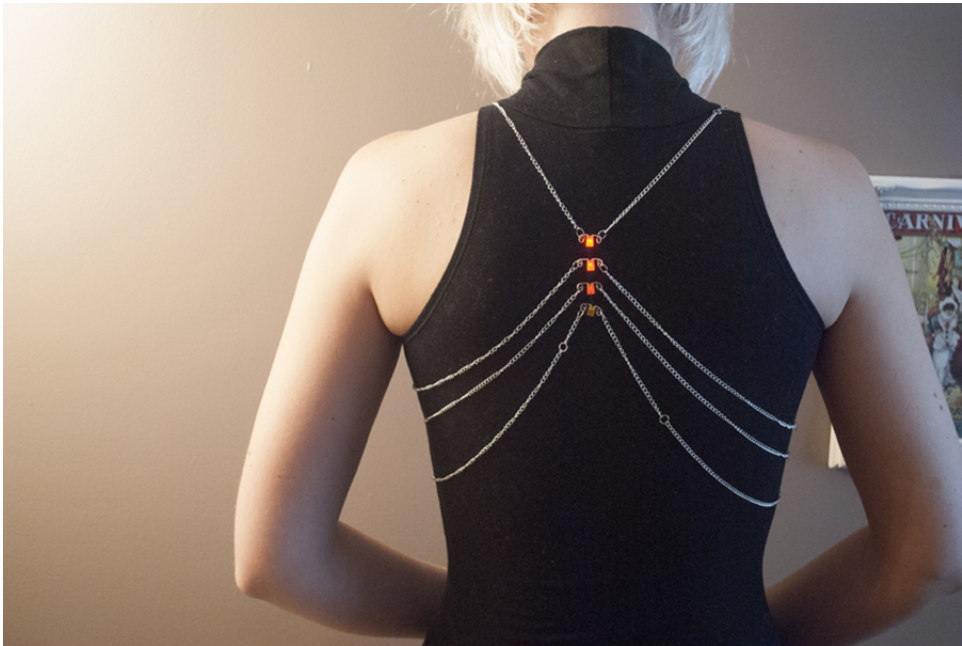
Figure 1-1. “Connection and Motion” by Izzie Colpitts-Campbell; this wearable circuit uses stainless-steel-coated brass chain to connect LEDs to a battery pack
