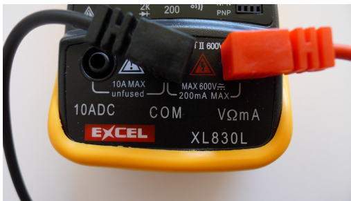
Figure 1-21. The connection for the probes; on this meter, you will need to move the red probe to the left if you are measuring current higher than 200mA
